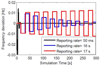
Case X - Analysis of the performance of the islanded operation controller considering the impact of data transmission delay
