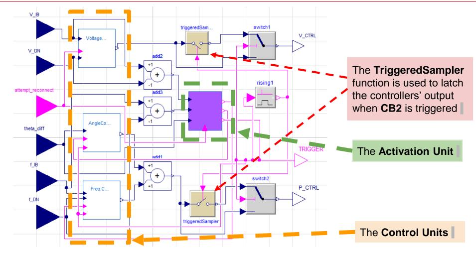
• The Boolean output signal from the re-synchronization unit is applied to the circuit breaker **CB2** when all three limits are satisfied
