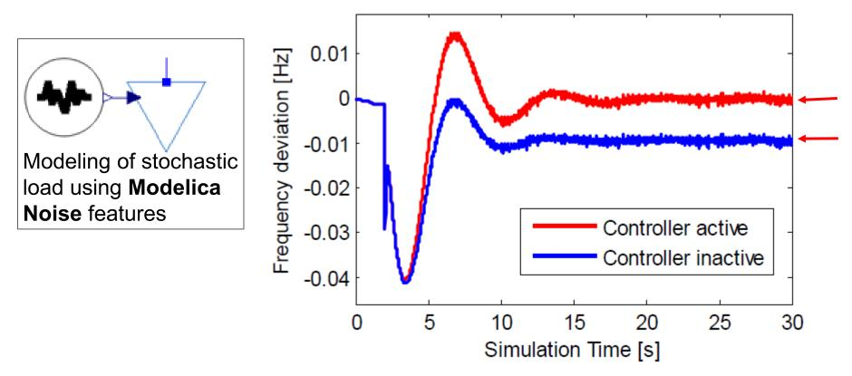
• The **stochastic load model** does not allow to accurately capture the frequency deviations due to time varying load changes. The controller is capable of reset the island's frequency to the prescribed reference in case of stochastic load.
