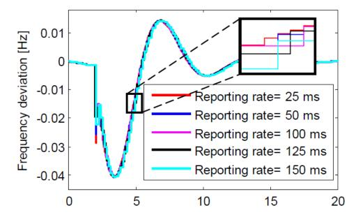
It is to observe that **delays** from **25 to 150 ms** have no major impact on the controller's performance, this is because the frequency dynamics being controlled are much larger than typical PMU reporting rates.
