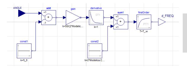
Modelica implementation of the Conventional WF-Based Freq. Computation Method (used in PSS/E, and all other power system simulation software)
