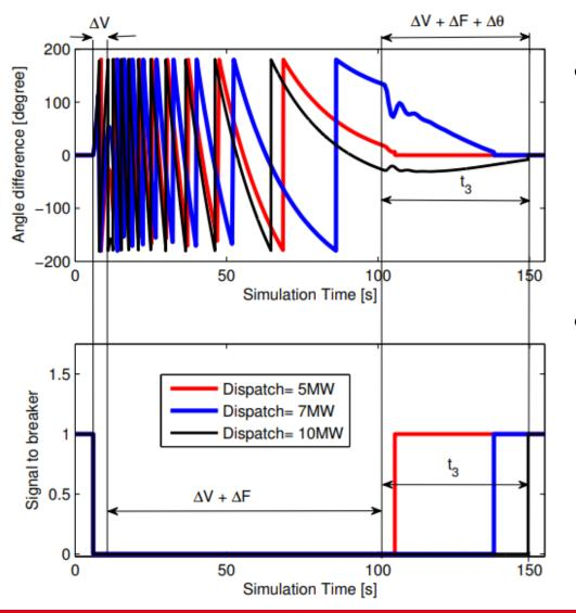
When the **angle difference** between the distribution and transmission network bus voltage phasors reaches a steady state value, **CB1** receives a **trigger signal** for automatic re-closure.
