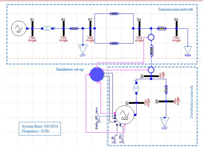
• The circuit breakers **CB1** and **CB2** are controlled using logic equations implemented in a **Simulation Set-up** block which is used to create the islanding event and to activate the islanded operation controller.
